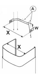
Adjust the width of the support bracket  ${\bf W}$  using screws  ${\bf A}.$  Fix the bracket to the ceiling or wall.
